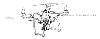
The Front LEDs glow solid red when the aircraft is turned on and help you orientate the aircraft when it is in the air. You can switch off the Front LEDs in the DJI GO app to achieve a better filming result. The Aircraft Status Indicators indicate the status of the flight controller. See the table below for details of its blinking patterns.
