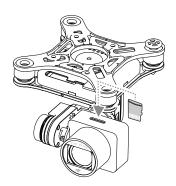
O DO NOT insert or remove the Micro SD card when the Phantom 3 Standard is turned on.
