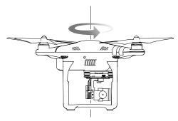
Hold the aircraft with its camera facing down, and rotate it 360 degrees along its central axis. The Aircraft Status Indicator will change from solid green to flashing yellow when complete. The calibration is successful.
