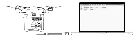
$\triangle$  The aircraft must be turned on in order to access the files on the Micro SD card.
